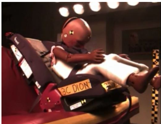
Figure 1. Example image of an ATD crash simulation for an upright child restraint system, such as the Merrit Wallenberg, Britax Booster, Diono Radian, and Graco Nautilus systems.
